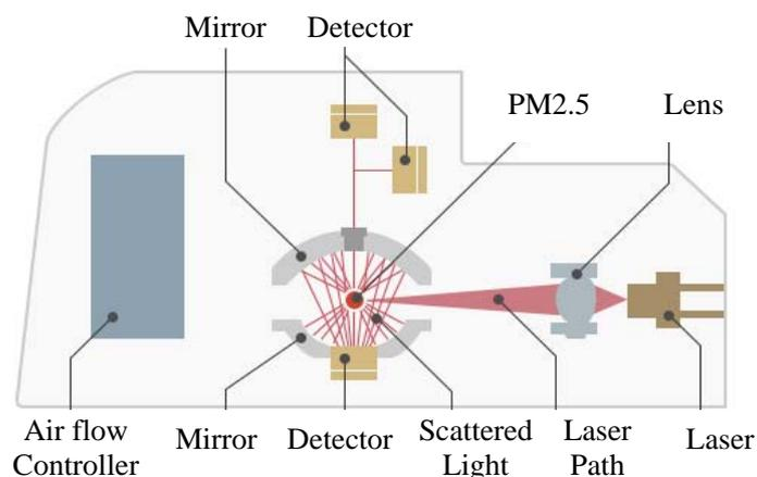
Structure of Air Quality Sensor (vertical cross-sectional view)
