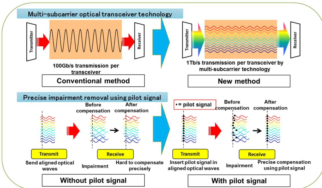
In optical communication, signals are carried on light waves known as carriers. Due to the limitation of signal bandwidth that can be generated without significant distortion, the throughput of a single carrier is also limited. Mitsubishi Electric achieved the 1Tb/s transmission rate with existing optical fibers by using a multi-subcarrier technology that transmits 11 light waves (subcarriers) simultaneously in a single channel by
