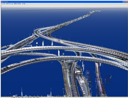
Example 2: Measurement of 3D junction with standard laser scanner superimposed with color camera images
