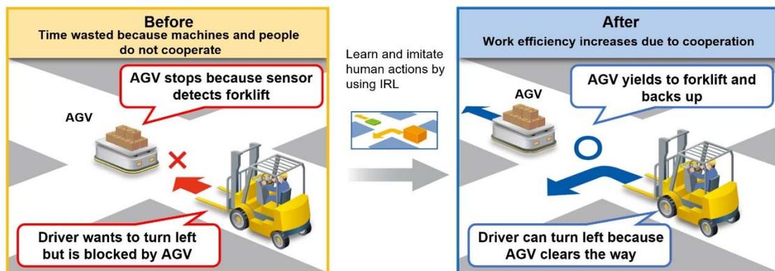
Example of cooperative AI deployed in AGV
