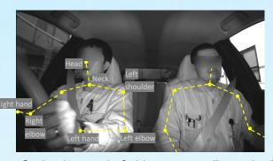
Optimal control of airbags according to body size
