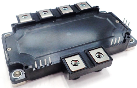
Dual switch (Half-Bridge)
