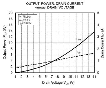
RoHS Compliance ,135-175MHz 8W 12.5V, 2 Stage Amp. For PORTABLE RADIO
