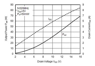
RoHS Compliance, 440-520MHz 30W 12.5V, 2 Stage Amp. For MOBILE RADIO
