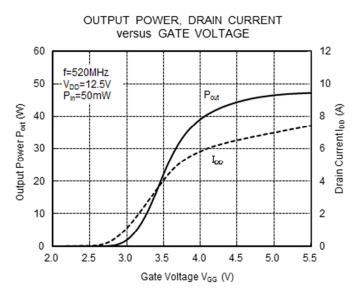
RoHS Compliance, 440-520MHz 30W 12.5V, 2 Stage Amp. For MOBILE RADIO
