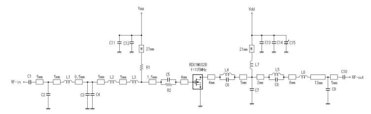
Note:Board material- Glass-Epoxy Substrate Micro strip line width=1.3mm/500HM,er:4.8,t=0.8mm W:Line width=1.0mm
