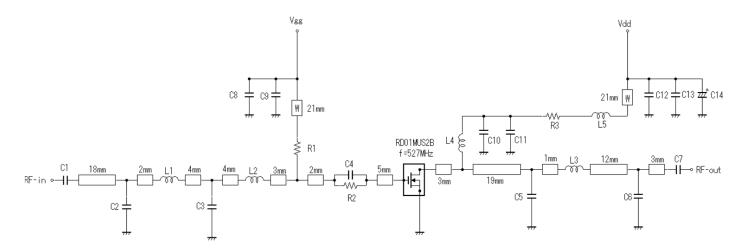
Note:Board material- Glass-Epoxy Substrate Micro strip line width=1.3mm/500HM,er:4.8,t=0.8mm W:Line width=1.0mm
