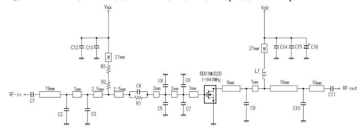
Note:Board material- Glass-Epoxy Substrate Micro strip line width=1.3mm/500HM,er:4.8,t=0.8mm W:Line width=1.0mm
