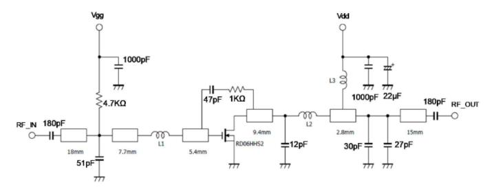
L1: Enameled wire 7Turns, D 0.23mm, O.D 1.62mm L2: Enameled wire 4Turns, D 0.23mm, O.D 1.62mm
