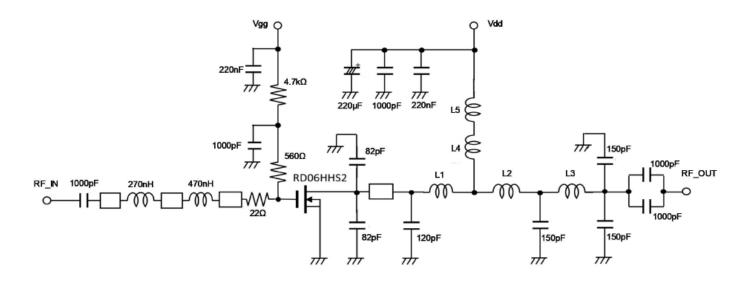
L1 : Enameled wire 6Turns, D 0.4mm, O.D 2.46mm L2 : Enameled wire 5Turns, D 0.4mm, O.D 2.46mm
