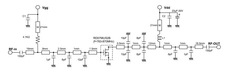
Note:Board material Glass-Epoxy substrate Micro strip line width=1.3mm/50 $\Omega$ ,er:4.8,t=0.8mm W:line width=1.0mm
