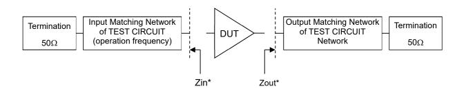
Zin\*: Input Matching Network impedance measured from DUT
