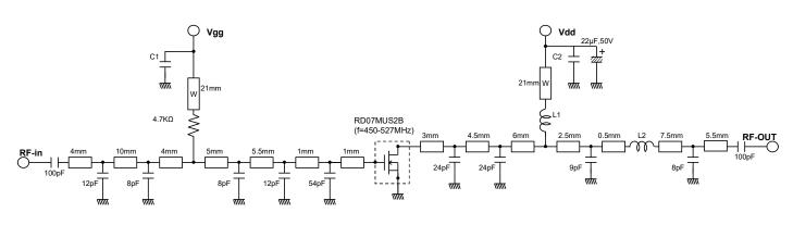
Note:Board material Glass-Epoxy substrate Micro strip line width=1.3mm/50 $\Omega$ ,er:4.8,t=0.8mm W:line width=1.0mm
