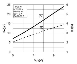
RoHS Compliance, Silicon MOSFET Power Transistor, 175MHz, 10W
