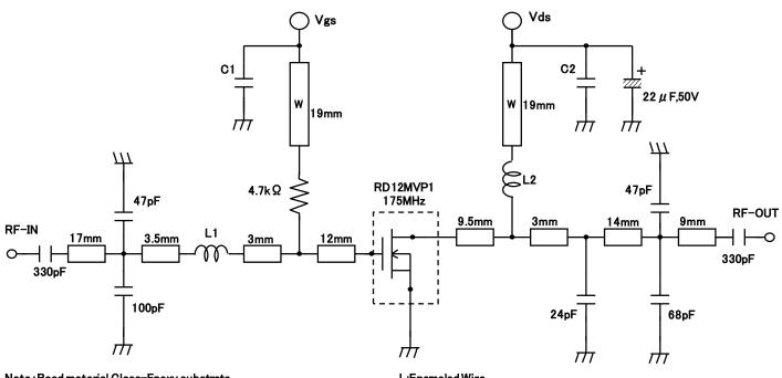
Note : Boad material Glass-Epoxy substrate Micro strip line width=1.3mm/50  $\,\Omega$  、er:4.8、t=0.8mm W : Line width=1.0mm
