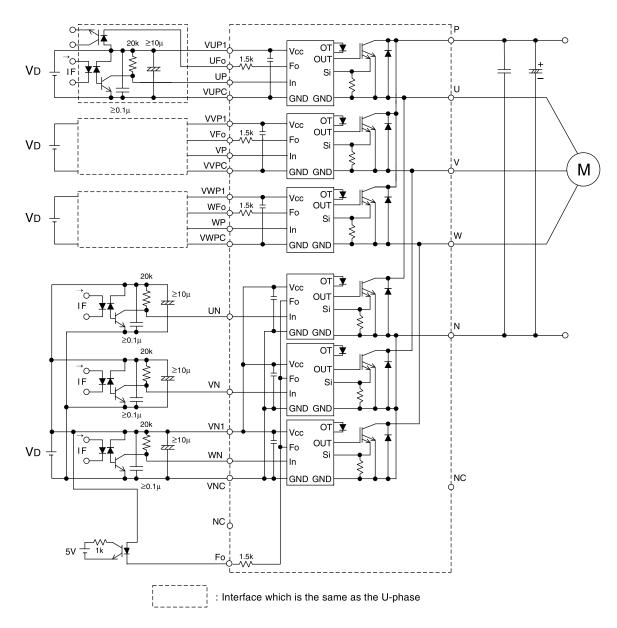
Fig. 8 Application Example Circuit
