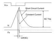
Fig. 6 SC Test Waveform
