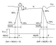
Fig. 4 Switching Time Test Waveform
