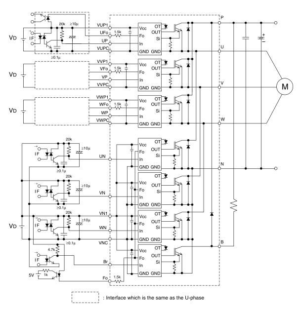
Fig. 8 Application Example Circuit
