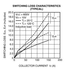
SWITCHING RECOVERY LOSS CHARACTERISTICS (TYPICAL)
