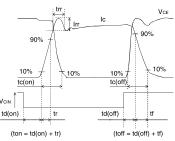
Fig. 4 Switching time test waveform
