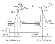
Fig. 4 Switching Time Test Waveform
