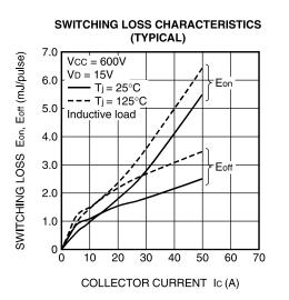
SWITCHING RECOVERY LOSS CHARACTERISTICS (TYPICAL)
