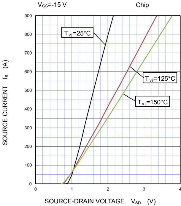
SOURCE-DRAIN ON STATE VOLTAGE
