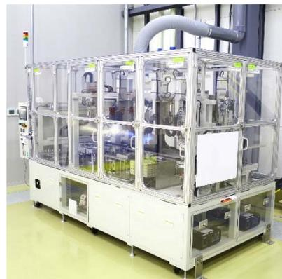
One-piece-flow automatic-sliding plating machine
