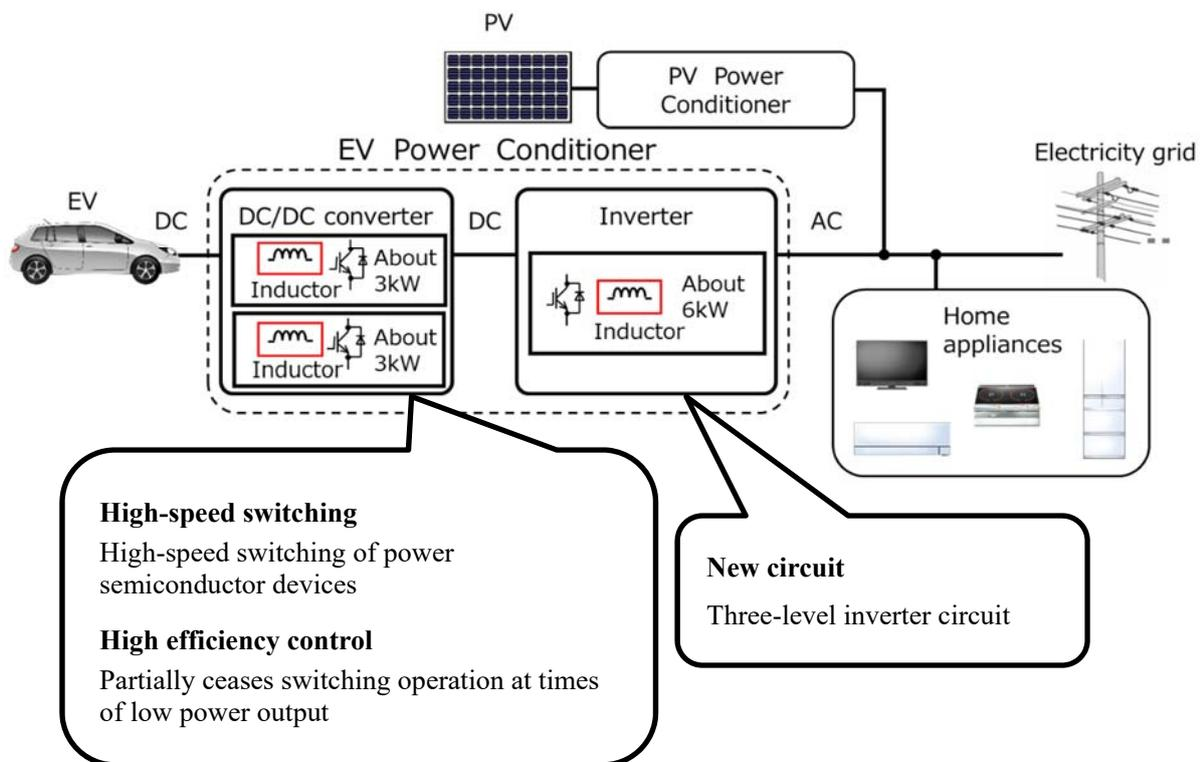
Fig. 2 Configuration of new EV power conditioner
