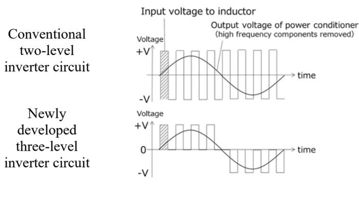
Fig. 4 Reduction in the amplitude of input voltage
