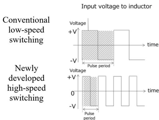
Fig. 3 Switching of power semiconductor devices
