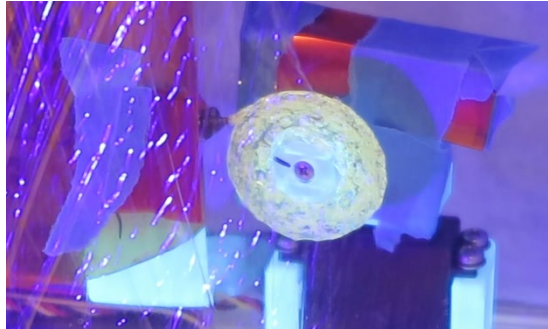
Mid-printing using an ultraviolet light source in a vacuum below 0.2kPa (Enlarged area around the nozzle and rotary axis motor)
